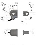
**Stainless Steel** Max. static load 5400 N Blueglobe connection
